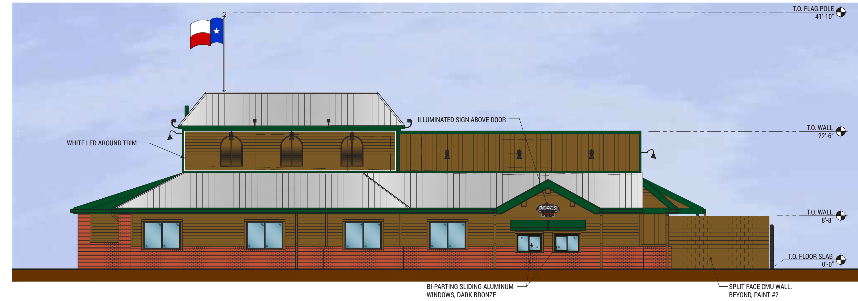
RIGHT ELEVATION (NORTHEAST)
